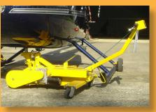
inclines. The design of the Helimover enables the operator to turn the helicopter though 360 degrees within its own length, enabling into wind departures every time, and easy confined space hangar manoeuvring
