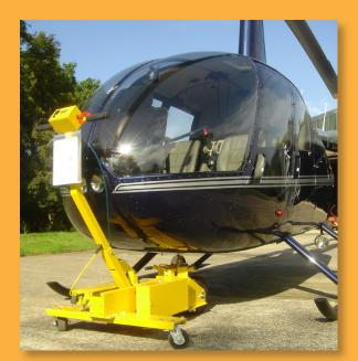
Fit the Robinson wheels and raise the skids. Then move the Helimover under the helicopter, push down on the handle to engage the ball hitch socket on the towing ball (already fitted to your R22, R44 or R66), and move the helicopter effortlessly.
