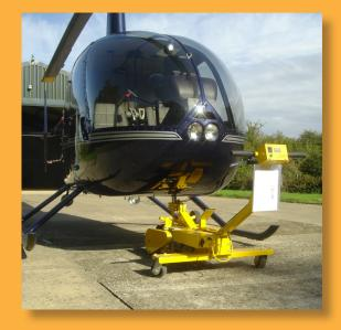
The Helimover<sup>™</sup> is an electric tug designed for Robinson R22, R44 and R66 helicopters. It provides a simple and economic means of ground handling for Robinson helicopter owners and operators.
