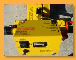
Forward/reverse direction and speed are controlled by a "wig wag" throttle and speed range selector mounted on the handle, with battery condition and diagnostic display. Soft start/stop.
