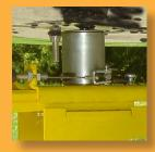
A clever locking balanced lever system moves the ball hitch socket upwards to capture, and lock onto, the Robinson tow ball.
